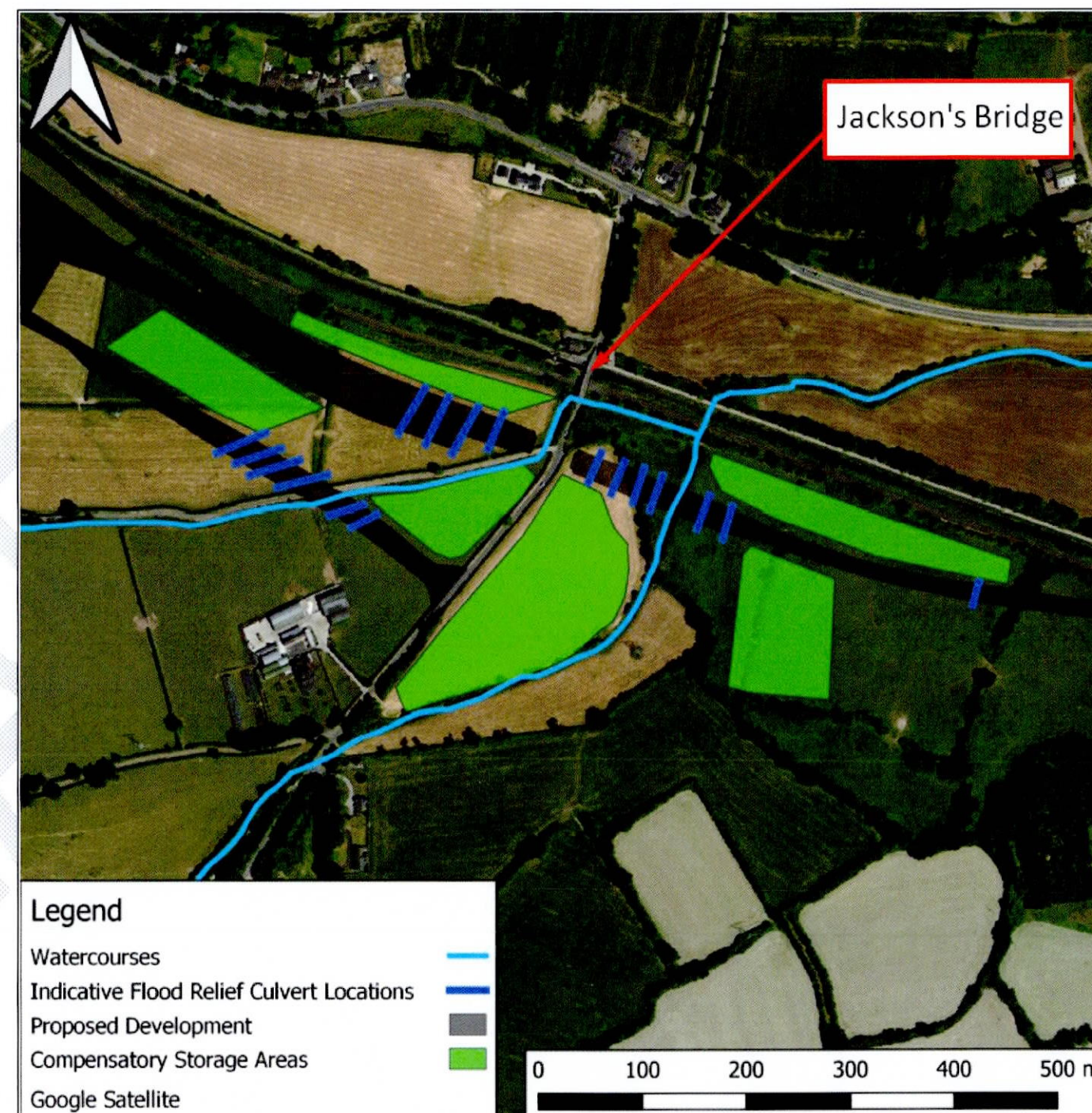
Figure 5.12: Map taken from DART + West SFRA Document showing the proposed Compensatory Storage Areas located south of Jackson's Bridge and directly above a vulnerable aquifer. (Source: DART + West SFRA Document, page 33, annotated by Tom Phillips + Associates, October 2022.)
